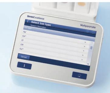
The twelve most commonly used ion types are pre-programmed in the instrument making the settings as convenient as possible. For others you can enter the ion charge and molar mass to ensure that all calculations and conversions are done for you.
