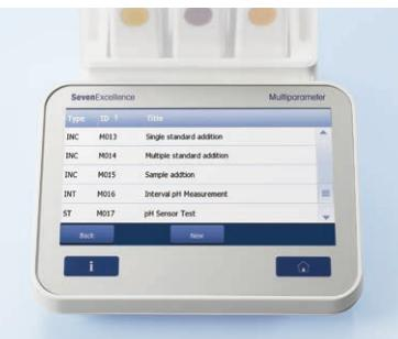
Special methods for the most common incremental ion measurements techniques are included, such as various standard addition/subtraction and sample addition/subtraction methods. This gives you a flexible and temporary tool kit for professional ion measurements!
